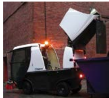
ABOVE CN100 Internal Fan & Airflow BELOW Stainless steel hopper gives 60" dumping height
