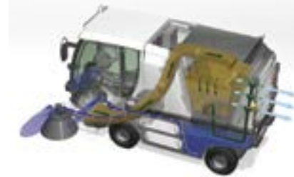
ABOVE CN100 Internal Fan & Airflow BELOW Stainless steel hopper gives 60" dumping height
